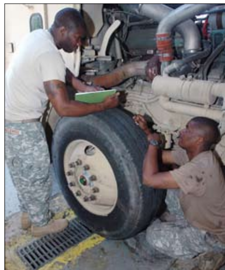
Photo by Staff Sgt. Roy Henry Sergeant 1st Class Junior Hazelwood (left) and fellow mechanic Staff Sgt. Garye Ware, talk over progress being made on adjusting the newly replaced front brakes of an 1148th Transportation Company semi tractor.
